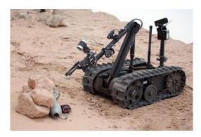
The suitcase portable robot is controlled through a two-way RF/F/O line from a portable or Wearable Operator Control Unit (OCU) that provides continuous data and video feedback for precise vehicle positioning.
